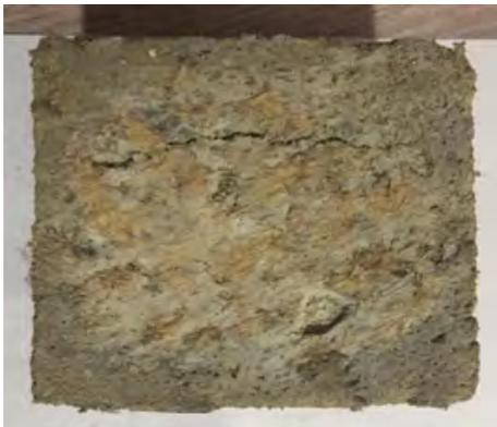
*Fig. 5 – Sawdust concrete of 1 mm fractional composition of sawdust*
