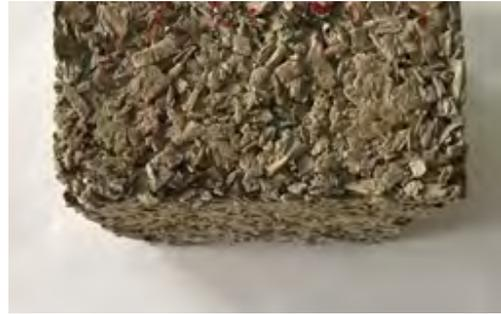
*Fig. 2 – Sawdust concrete of 5 mm fractional composition of sawdust*
