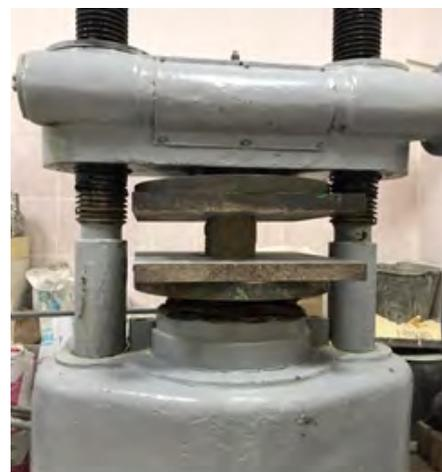
*Fig. 6 – PSU-10 hydraulic press*
