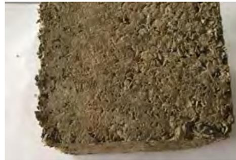
*Fig. 4 – Sawdust concrete of 3-1 mm fractional composition of sawdust*
