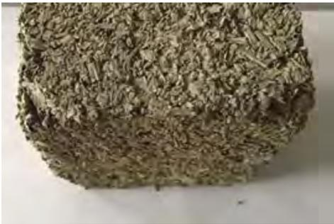
*Fig. 3 – Sawdust concrete of 5-3 mm fractional composition of sawdust*
